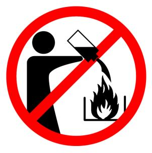
1. SHUT BURNER OFF WITH DAMPENER/SLIDER OR PROVIDED SNUFFER TOOL FOR CUPS OR ALLOW FUEL TO BURN OUT COMPLETELY. ALLOW 30 MINUTES FOR UNIT TO COOL BEFORE REFUELING.
